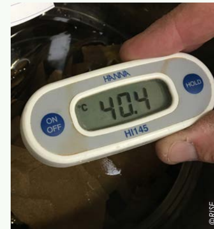
Temperature check during repulping
