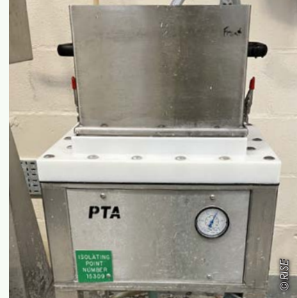
The Somerville Fractionator houses the coarse or fine screen to facilitate separation of fibres from rejects. The fibres are made into hand sheets to assess the properties of the paper.
